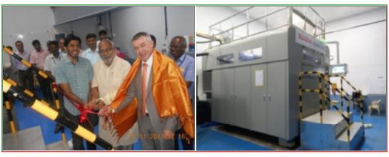
Magna can now offer Rapid Casting Development through its Tool Less Development of Castings, Cores and Molds utilizing Sand 3D printing technology. The maximum size of the molds/ cores are 1500mmx1000mmx750mm. The process uses special imported sand and resins for the manufacture of the Molds and Cores. The facility has been in operation from January 2018 and has built up a wide range of customers and products. Examples of which are as follows:
